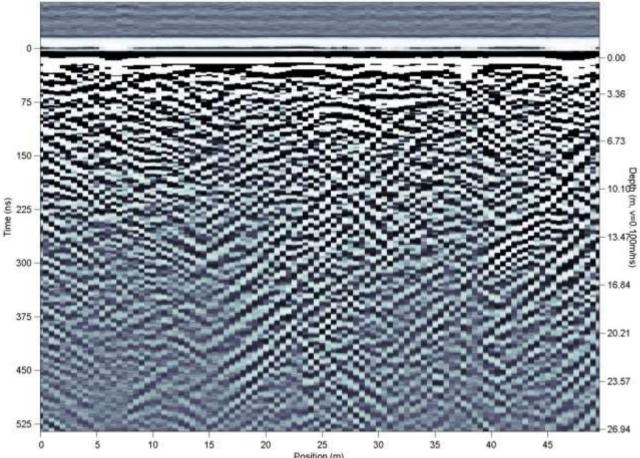
Position (m) Figure 61: GeoRadar profile recorded at site B. Each vertical trace represents one measurement along the profile. An example of a reflection is seen 3.4 m below the surface and 25 m from the start of the profile. The magnetic anomaly was caused by something 10-15 below the surface. The reflection therefore cannot be the same object that caused the magnetic anomaly.
