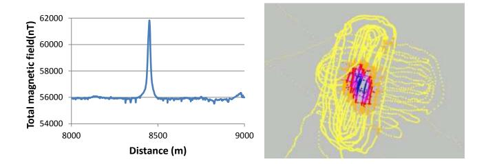
Figure 60: a) Profile showing the intensity of the magnetic field along a profile mapped at Site B on Meteorite Island. b) Color coded magnetic field measurements at the same location as a). The field strength increases from 56000 nt (Yellow) to 61000 (dark blue)
